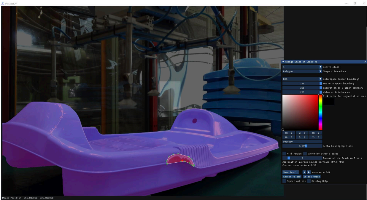
Labeling of an injection molded part with defect type short shot defect for semantic segmentation
