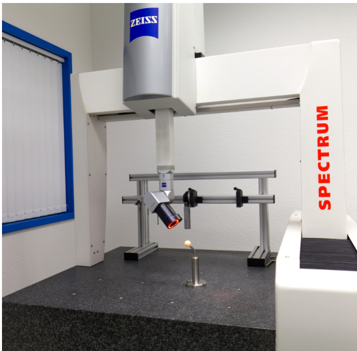
Video-optical sensor ViSCAN Multi-sensor coordinate measuring machine SPECTRUM from Carl Zeiss Oberkochen
