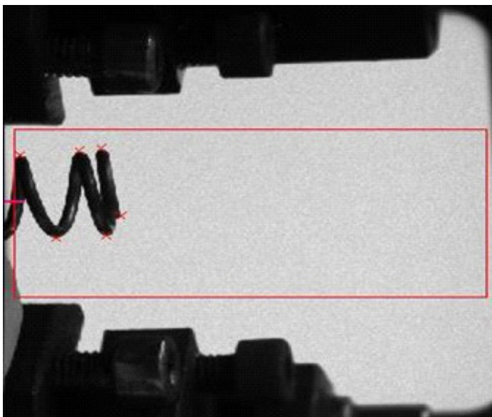
Oscillating spring in the machine with automatic tracking of the measuring points
