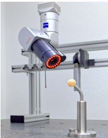
RingLight on the Zeiss Viscan for precision measurements
